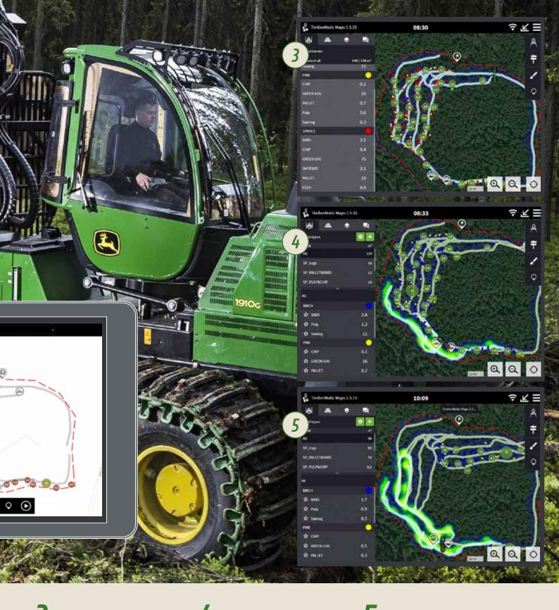
The harvester operator can see exact job-site boundaries and the amount of harvested timber. He can also mark special instructions, like the locations of fuel tanks or difficult spots for the forwarder (ditches, pits, rocks etc.).
