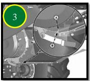
The cob deflector #1 should be in the up/small grain position. The vanes in the rear deflector or the chop to drop door #2 can be adjusted to further improve the residue distribution.
