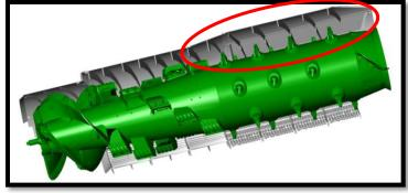
The rotor top covers should be in the standard position and only placed in the advanced position if you want to improve the straw quality since this will reduce separation slightly.
