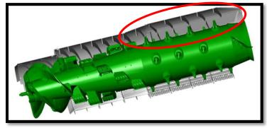
The rotor top covers should be in the standard position and only placed in the advanced position if you want to try to reduce the material on the cleaning shoe.
