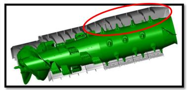
The rotor top covers should be in the standard position and in very dry conditions it could help reducing the shoe load setting the vanes to advanced.
