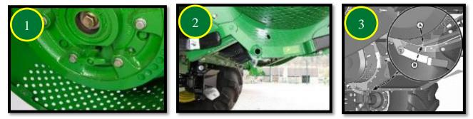
The cob deflector #1 should be in the up/small grain position. The vanes in the rear deflector or the chop to drop door #2 can be adjusted to further improve the residue distribution.
