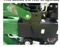
**Reel is not level** Rephase Reel by lowering it completely. Table must be in rear position, reel fully extended. Bleeding is not required.
