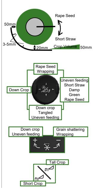
In Short Crops do not retract the Cutter bar shorter than 450mm. Also extend the table first completely and then retract it. Doing this the sealing bridge will be moved all the way forward. This will allow you to have the Reel in a better position to sweep the Cutterbar and move material to the Auger
