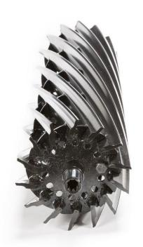
At John Deere, we're committed to providing hardworking, long-lasting parts for your operation. That's why we created our **14 Blade Reel**. This reel offers the ability to lower your frequency of clip, which is defined by the distance traveled between consecutive cuts. By lowering the frequency of clip, you can produce a smooth, clean cut that increases the playability of the putting surface.
